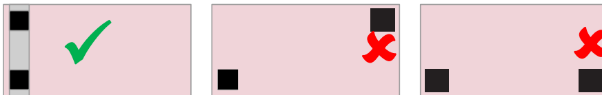
Fig. 6: Recommended barcode placement for large items
