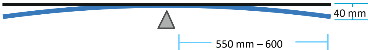
Fig. 31: Maximum permissible cardboard deformation due to suction force of the depalletiser
