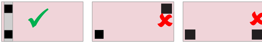
Fig. 6: Recommended barcode placement for large items
